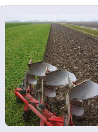
Agrometius, the Dutch distributor of Trimble AgGPS<sup>™</sup> products has developed a system to control vari-ploughs with RTK-GPS. The **GeoPlough 100 system** adjusts the plough width hydraulically according to the offline distance. This way a curved furrow can easily be made straight. Geoplough 100 is an "add on" for tractors which are equipped with the Trimble Autopilot system.
