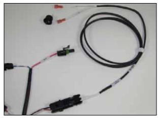
Step 3 Connect the R7 cable to the switch pins. Note - Polarity is not important.
