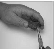
1. Grasp the crimped contact approximately one inch behind the contact barrel.
