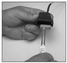
3. Remove the plastic inserts from the location where you will insert wires/pins.
