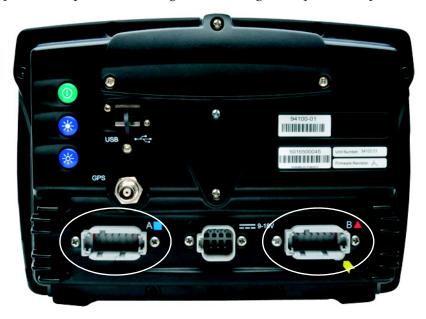
The replicator port on most cables breaks away the pins not used by the primary device the cable was designed for.
